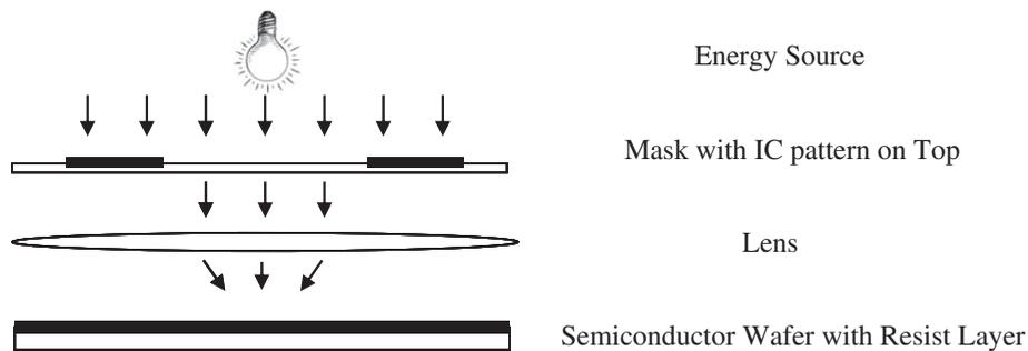
Figure 3. Basic principle of the semiconductor lithography process
